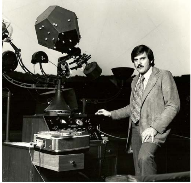
Figure 2. Author poses with the audio and video systems added to the planetarium capability during the 1970s. Shown is the Spitz A-2 primary and auxiliary projectors that were situated on the control console in the center of the planetarium chamber.
